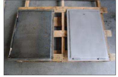
*A before and after comparison of tightly adherent mill scale being blasted to an SSPC-SP 5 White Metal.*
