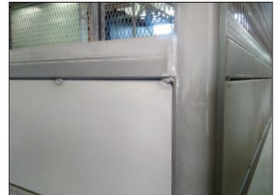
*Here is an example of mill scale staining on tube and blasting to a White Metal on cold rolled steel.*
