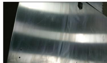
*This is an example of how not to solvent wipe a product before coating. The streaks on the surface are residual oil from solvent wiping.*
